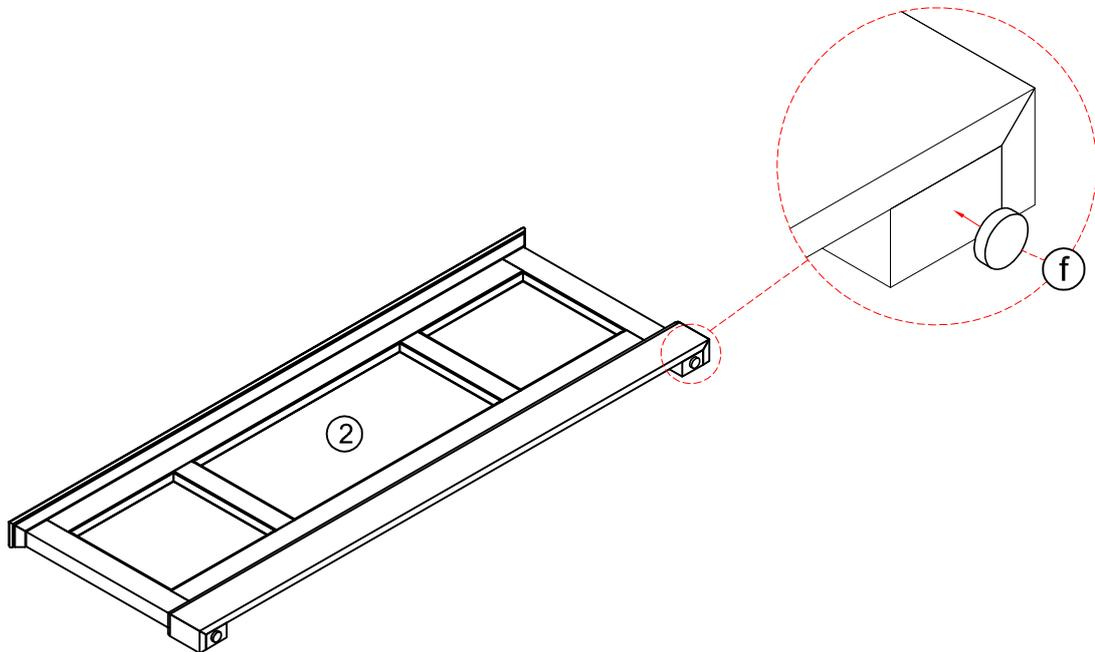
STEP 2: Attach side rails ③ to headboard legs ① and footboard ② by interlocking the brackets on the side rail with the bolt ④ on the headboard/footboard and then push down to lock in place.
